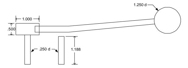
Figure 7, Turning Handle with Top and Bottom Pivot
