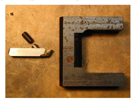
The clearance slot is located by inserting a new bit and scribing the top/bottom of the slot. Add an additional 50 thousandths for kicks and for any wear on the thrust bearing that will drop the cutting bit down.
