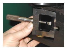
The micrometer head was turned down only as much as needed and the hole in the housing is bored to the micrometer head diameter plus 0.002" for the Locktite.
