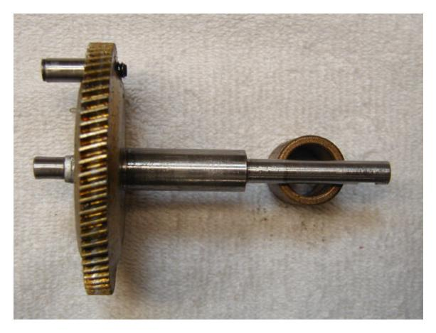
The assembled adjustable stop plate picture is below. I made two adjustable stops. In practice, only one is needed. The plate rotates and sets the starting point at the end of the stop slot. The ending point is then set with the adjustable stop.
