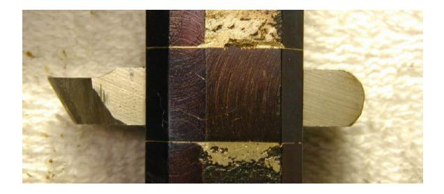
Next a hole for a  $\frac{1}{4}$  x 28 set screw was drilled and tapped. Note the thread portion is not tapped through (bottom tapped) in the drawing to ensure a non-threaded surface for the angled plug.
