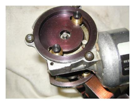
Note the stop plate is machined to the outside diameter to accommodate the use of cap screws to lock the plate down. The original tapped holes were just slightly in the wrong place. The new tap drill diameter holes were located with a rotary table, milled with a boring head, and tapped. An alternative would be to change the design of the outer edge of the adjustable stop plate to fit the existing holes.
