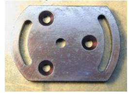
An adjustable stop plate was fabricated to mount on the top of the gearbox, as one can never have enough features. The following are pictures of the top and bottom views of the adjustable stop plate.
