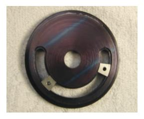
The T-nuts were milled out with the correct radius for the slot. They would probably be fine with parallel sides, but they fit and slide quite well with the mating curved sides.
