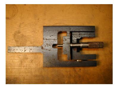
Machining the Yokes' Holes: The bushing, setscrew, and pivot holes were located via the mill table and should be drilled/reamed before turning the bushings. The bottom bushing proves the thrust surface for the downward cutting pressure and the top bushing is a simple cylinder. The bushings are turned and pressed in. The gap between the top of the Swiveling Yoke and the bottom of the Frame Yoke is insignificant and left alone. One could refine the design and eliminate the gap.
