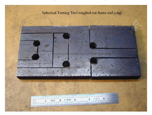
Three pieces were used, picture below. The two yoke pieces were milled to spec cleaning up all edges except the mill scale. The clearance slot in the Frame Yoke was milled later. Additional clearance milling (beveling) on the Swiveling Yoke was preformed to increase the swiveling range.
