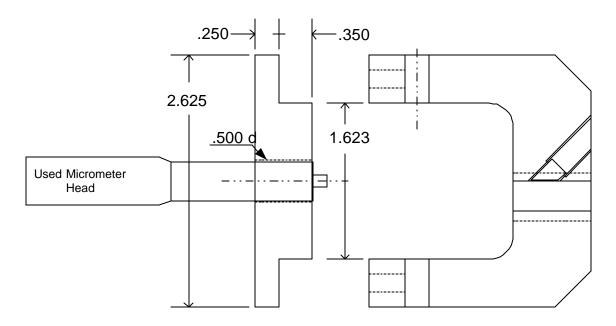
Figure 8, Micrometer Bit Setting Tool
